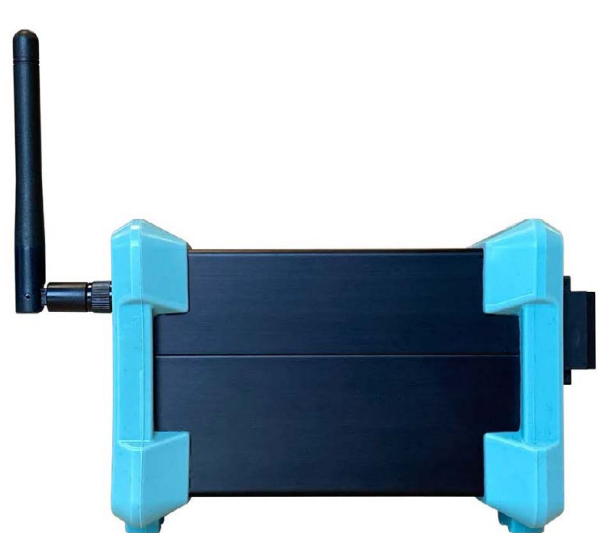
dydaqmeas with 8 analogue inputs, digital I/O and a powerful ARM ® CPU
