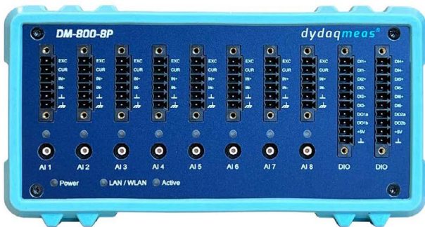
dydaqmeas with 8 analogue inputs, digital I/O and a powerful ARM ® CPU
