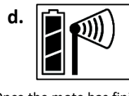
Once the mote has finished joining the network, the "x" icon is removed and the channel count on the station LCD increases by three (two for soil moisture and temperature, and one for the mote battery).
